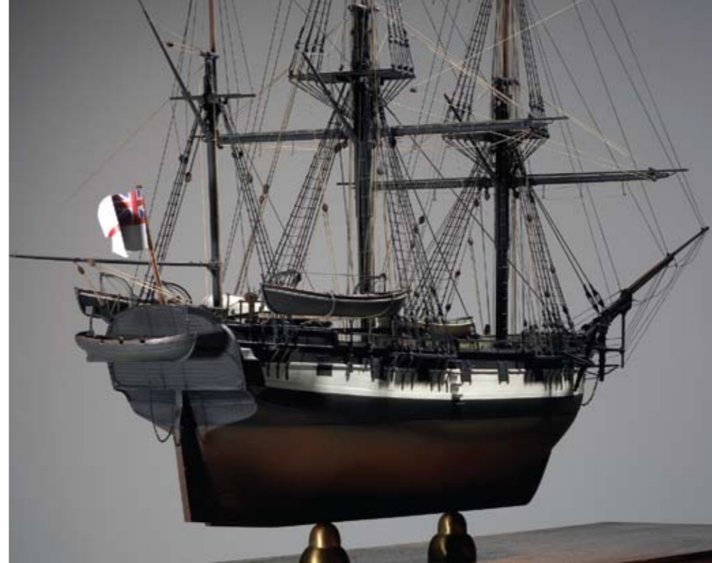
Completed model of one of history's most famous ships of scientific discovery, HMS Beagle , by Mike Bass of Cutting Edge Models. Launched in 1820 as a brig, Beagle was later refitted for survey. A mizzen mast was added, and for Darwin's voyage a poop cabin and forecabin were built. Photographer A Frolows/ANMM
